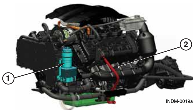
Figure 7.4 – Oil Filter and Drain
