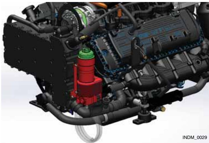
Figure 3.3 – Engine Oil Cartridge Filter
