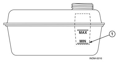
Figure 7.6 - High Fill Tank
