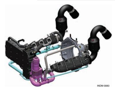
Figure 8.1 – Raw Water Cooling System
