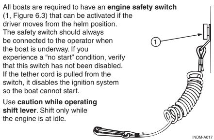
Figure 6.3 – Typical Tether Cord and Safety Switch
