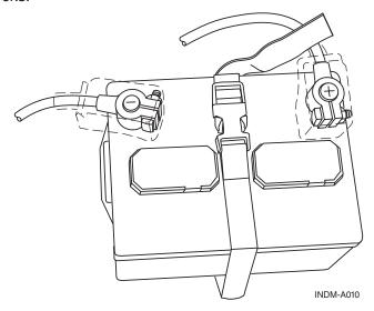
Figure 3.4 – Battery Connections
