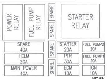
Figure 7.8 – Fuse Box Layout
