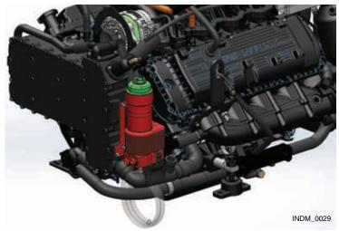
Figure 3.3 – Engine Oil Cartridge Filter
