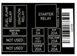
Figure 7.7 – Fuse Box Layout
