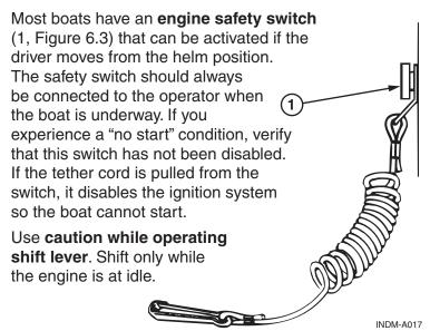
Figure 6.3 – Typical Tether Cord and Safety Switch
