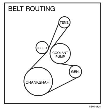
Figure 7.8 – Serpentine Belt Routing
