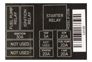
Figure 7.7 – Fuse Box Layout
