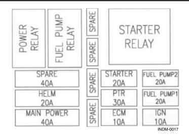
Figure 7.14 – Fuse Box Layout
