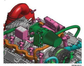
Figure 7.5 – Flame Arrestor
