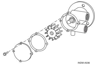
Figure 7.8 – Raw Water Pump Impeller
