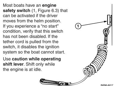
Figure 6.3 – Typical Tether Cord and Safety Switch
