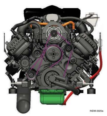
Figure 7.15 – Serpentine Belt Routing
