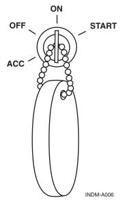
Figure 4.1 - Engine "On" Switch
