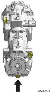
Figure 8.6 - Indmar-Vee Through Shaft Drain Plug
