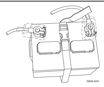
Figure 3.5 – Battery Connections
