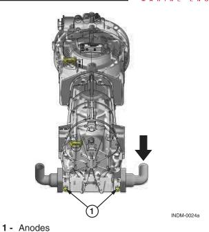
Figure 8.3 – ZF Ski-Vee Water Drains
