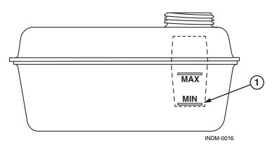
Figure 7.6 – High Fill Tank
