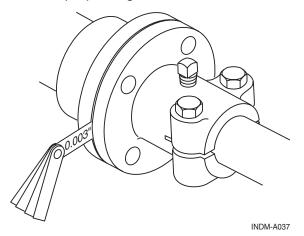
Figure 8.8 – Prop Shaft Flange Alignment
