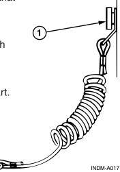
Figure 6.3 – Typical Tether Cord and Safety Switch
