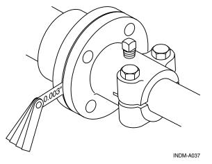
Figure 8.7 – Prop Shaft Flange Alignment
