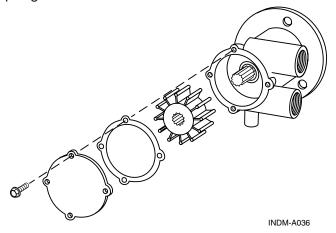
Figure 7.9 – Raw Water Pump Impeller
