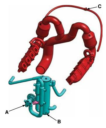
Figure 8.1 – Cooling System Draining
