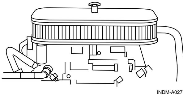
**Figure 6.5 – Flame Arrestor**
