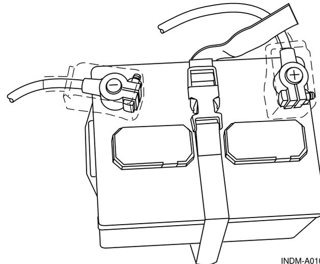
**Figure 2.4 – Battery Connections**
