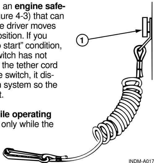
**Figure 4.3 – Tether Cord and Safety Switch**
