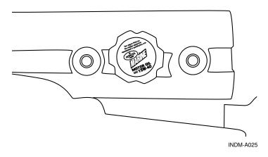
Figure 6.3 – Engine Oil Fill
