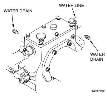
Figure 7.4 – V-Drive Drain Plugs
