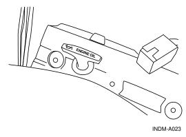
Figure 6.1 - Engine Oil Dipstick Location
