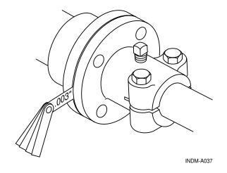
Figure 7.5 – Prop Shaft Flange Alignment
