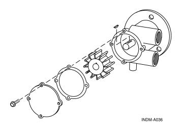
Figure 7.2 – Raw Water Pump Impeller
