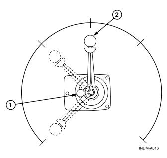
Figure 3.4 – Shift/Throttle Lever
