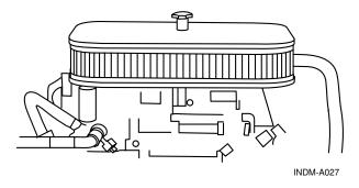
Figure 6.5 – Flame Arrestor
