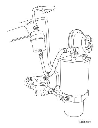
Figure 5.2 – Inspecting Fuel Lines
