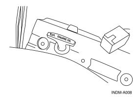
Figure 2.2 – Engine Oil Dipstick
