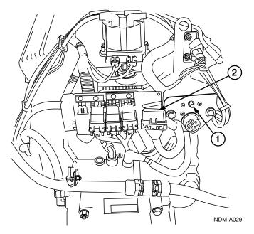
Figure 6.10 - Breaker Reset Button
